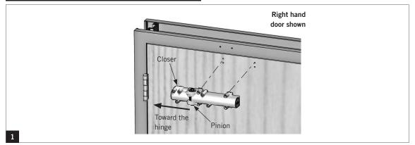
NOTE: Orient pinion closest to hinge.
