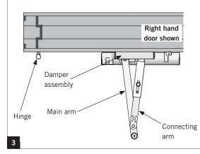
3.1 Slide end of connecting arm into end of damper assembly.
