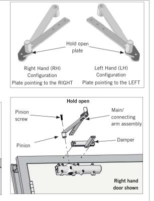
NOTE: To disassemble hold open plate:
