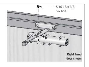
3.2 Secure connecting arm and damper assembly.
